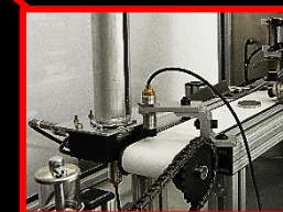
PART MAGAZINE, PART LOADER, PROXIMITY & MAGNETIC SENSORS, AND PNEUMATIC ACTUATORS
